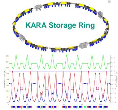
Extended DBA lattice (dispersion>0 in straight section) Designed emittance = 59 nm-rad
